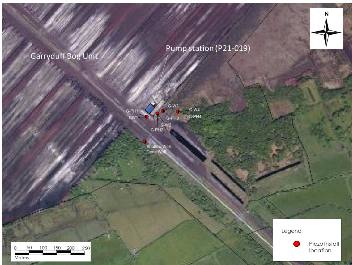
Figure E: Garryduff - piezometer install location map
